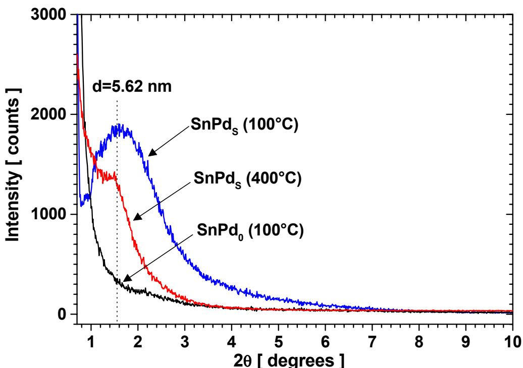
**Fig. S1.** Low angle XRD of  $\text{SnPd}_s$  films deposited on Corning 7059 glass substrates. The low angle XRD of the corresponding  $\text{SnPd}_0$  film prepared without surfactant is also shown.
