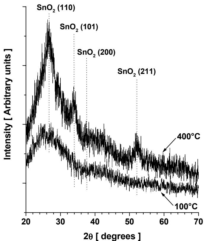
**Fig. S2.** The wide angle XRD of SnPds films deposited on Corning 7059 glass substrates heated at 100 and 400 °C. The 400 °C film shows broad peaks corresponding to cassiterite  $\text{SnO}_2$  structure. The  $\text{SnO}_2$  (101) peak overlaps with broad amorphous peak arising from the glass substrate.
