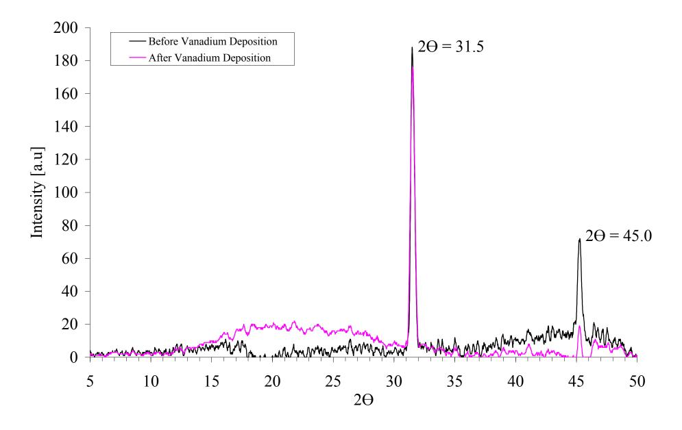
**Figure 1** - Wide angle powder XRD-pattern of the P/F resin before and after vanadium deposition. The patterns are characteristic for amorphous carbon frameworks.
