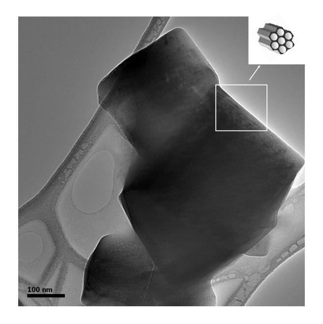
**Figure 4** - TEM image of mesoporous P/F resin calcined at 350°C
