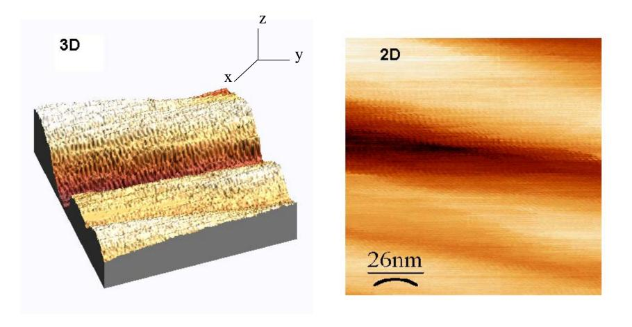
**Figure 5** – 3D and 2D AFM images of mesoporous P/F resin calcined at 350°C
