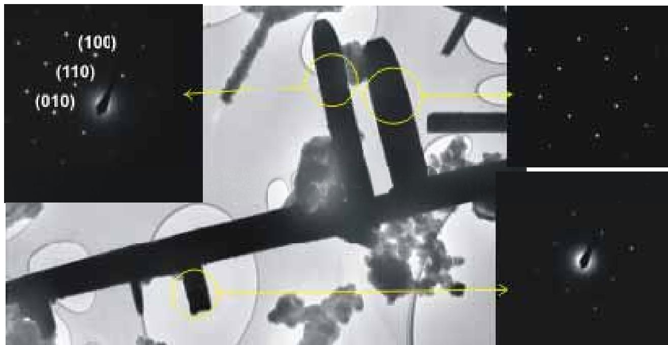
**Figure S7:** TEM images of Cu<sub>2</sub>O@PPy core/shell branched structures before (A & B) and after (A' & B') prolonged exposure to an intense electron beam.
