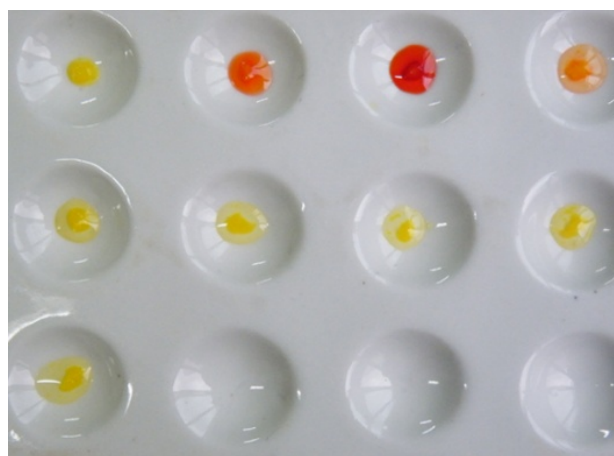
Fig. S4 Color changes observed upon the addition of various anions (10 mM) to DMF gel of F3 (15.6 mM, 1.0 wt %). From left to right: free F3 , F3 +F - , F3 +AcO - , F3 +H 2 PO 4 - , F3 +Cl - , F3 +Br - , F3 +I - , F3 +ClO 4 - , F3 +HSO 4 - .
