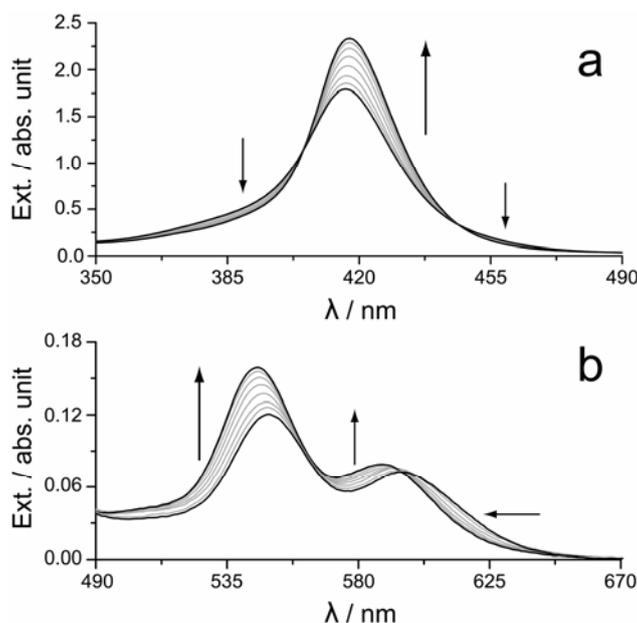
**Figure S1.** UV/vis extinction spectra of t-CuP in MilliQ water (8  $\mu$ M; a: Soret band, b: Q-bands), as a function of increasing temperature (from 10°C to 70°C, marked by arrows). The presence of several isosbestic points suggests there are only two chromophores present under these conditions.
