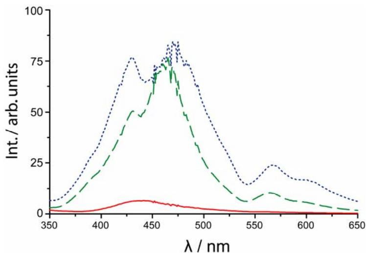
**Figure S4.** RLS spectra of t-CuP in the presence of PLG (pH = 4.58, solid; pH = 5.5, dotted; pH = 6.86, dashed), at high ionic strength. [t-CuP] = 5  $\mu$ M; [Glu] = 500  $\mu$ M, FW ~ 17 kD; [buffer] = 2 mM; [NaCl] = 0.15 M.
