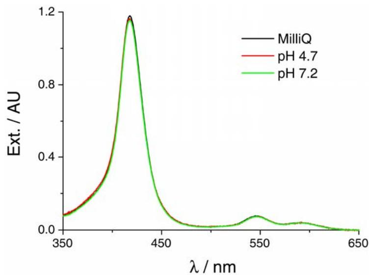
**Figure S2.** UV/vis extinction spectra of 5  $\mu$ M t-CuP in MilliQ water (black), pH 4.7 acetate buffer (red), and phosphate buffer (green), showing that under the ionic strength conditions (IS = 2 mM) used in the various experiment the presence of the buffers has a negligible effect on the porphyrin extinction features.
