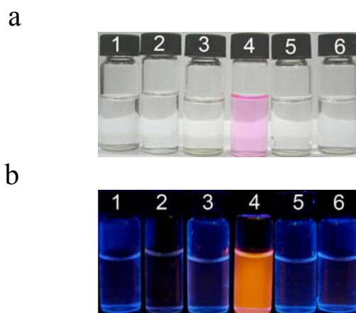
Figure S3. Color changes of probe 1 (10 \mu\text{M} ) in the presence of 5 equiv. of various species in 20 mM HEPES buffer, pH 7.4, containing 40% \text{CH}_3\text{CN} as a co-solvent. 1: free, 2: \text{Fe}^{3+} , 3: \text{H}_2\text{O}_2 , 4: \text{Cu}^{2+} , 5: \text{F}^- , 6: \text{Co}^{2+} : (a) visible color and (b) visual fluorescence color on excitation at 365 nm using a handheld UV lamp.
