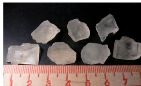
**Figure S1.** Morphology of crystals obtained from crystallization of *dl*-**1** from EtOAc solution. Scale in cm.
