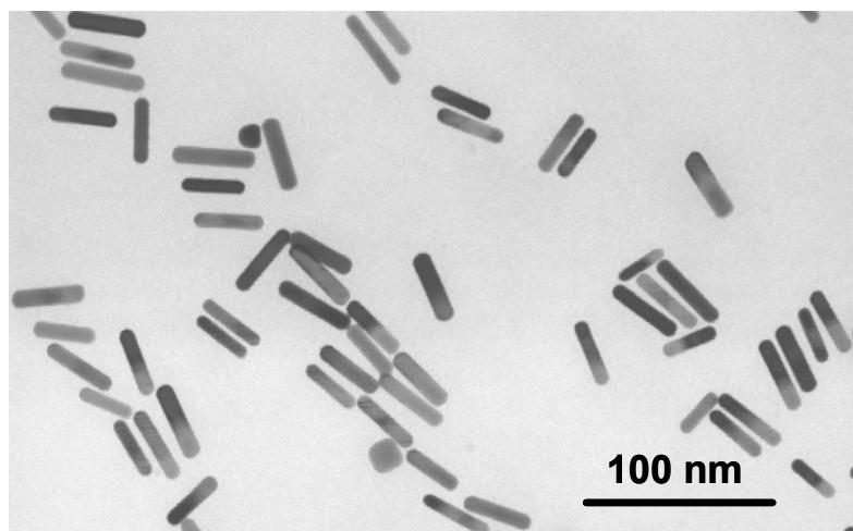
**Figure S1.** Transmission electron microscopy image of gold nanorods end-terminated with thiol-terminated polystyrene.
