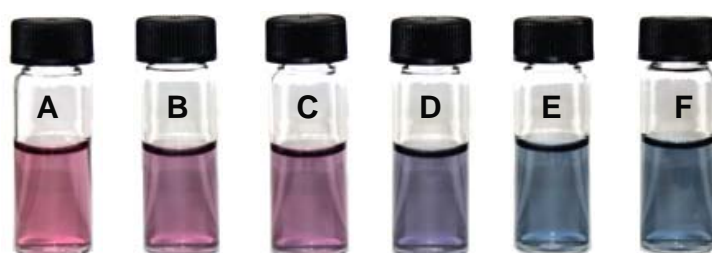
Fig. S4. Color change of cysteine-modified Au NPs reacting with different concentrations of triphosgene: (A) 0, (B) 10, (C) 20, (D) 25, (E) 30, and (F) 40 μM.
