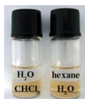
Fig. S5 Photograph of \text{Mn}_{12}\text{-C}_{18}/\text{C}_{18}\text{EO}_{10} aqueous solution extracted by chloroform and n -hexane.
