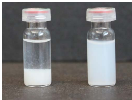
Fig. S5 Sedimentation of the click-conjugated particles (left) and the non-conjugated particles (right). The image was taken after the particle suspensions have been left to stand for 1 min. Total particle concentration: 4 \text{ mg mL}^{-1} in acetonitrile.
