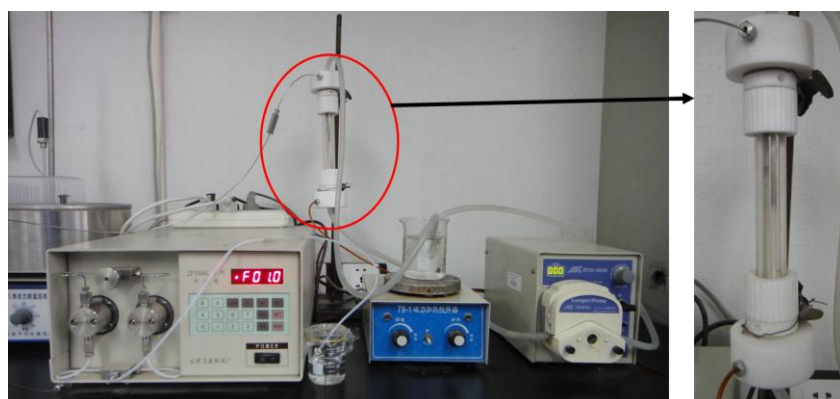
Figure S1: The digital photos of MDC device. The right photo is the ceramic membrane reactor composed of four ceramic membrane tubes [1], which is the core of the device of MDC method.
