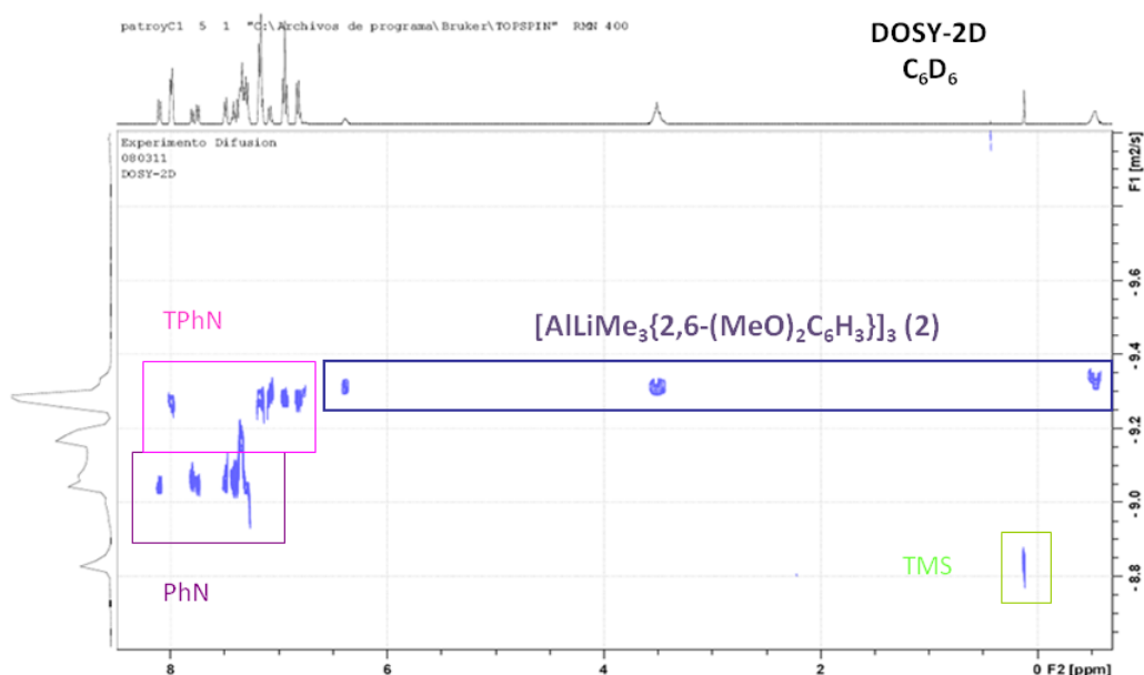
Figure 8. 2D DOSY NMR experiment of the mixture of TMS, PhN, TPhN and 2 in \text{C}_6\text{D}_6 . The x- and y-axis represent the regular ^1\text{H} chemical shift and the relative diffusion rate, respectively.
