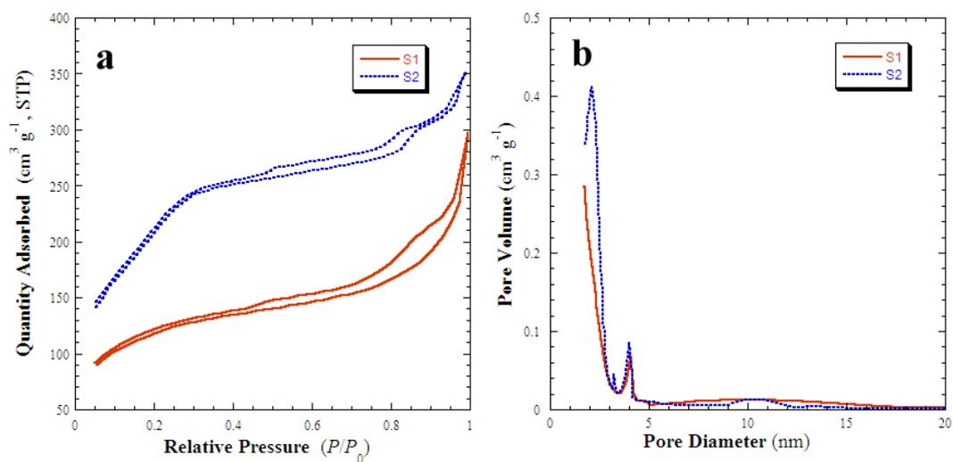
**Figure S3.** Sorption isotherms (a) and BJH pore size distribution (b) of the 4,4'-biphenylene-silicas, **S1** and **S2**. The sorption isotherms were determined by N<sub>2</sub> sorption-desorption measurements, and the pore size distributions were evaluated from the desorption branches.
