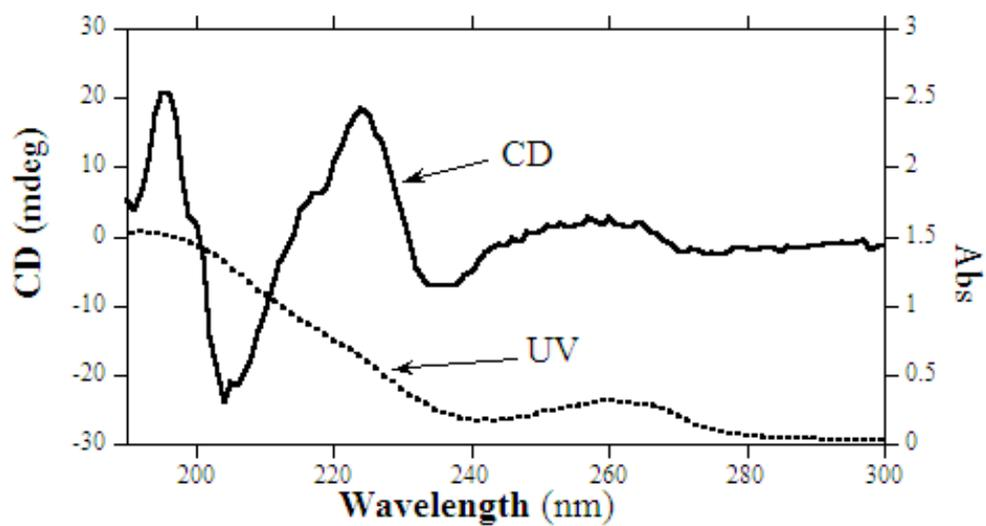
**Figure S1.** CD and UV spectra of L-18Phg4PyBr hydrogel.
