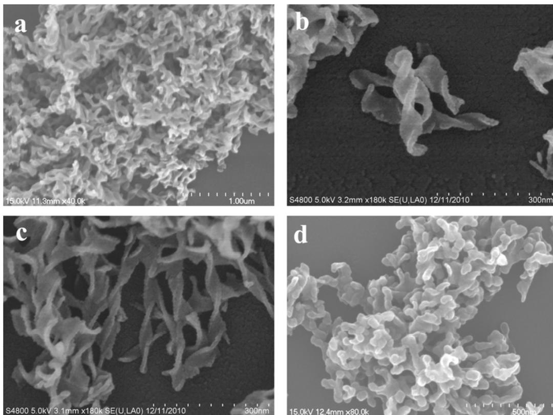
**Figure S4.** FESEM images of the samples (a) CS0, (b) CS1, (c) CS10, and (d) CS100.
