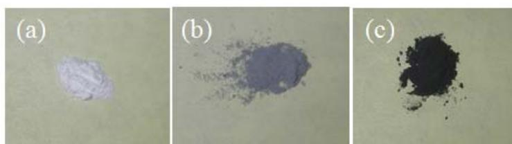
**Fig.S1** Photographs of the pure SL powder before (a) and after (b) c-MWNT coating.
