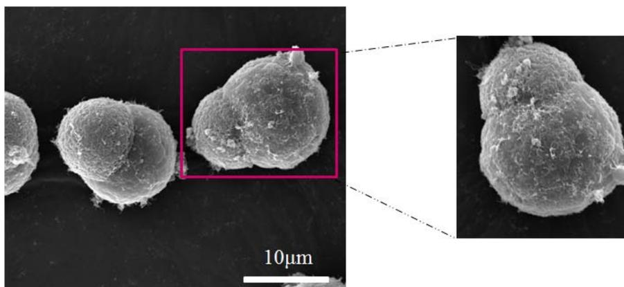
**Fig.S2** SEM images c-MWNT (5.65wt %) adsorbed SL particles.
