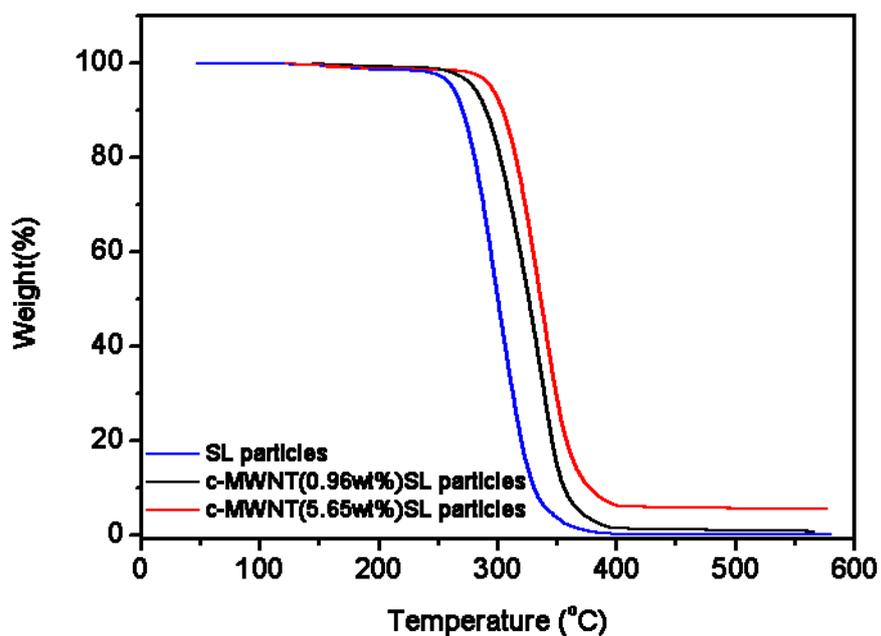
**Fig.S3**TGA curves of pure SL particles and c-MWNT adsorbed SL particles.
