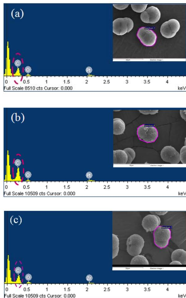
**Fig.S4** EDS spectrum of pure SL particles (a), c-MWNT adsorbed SL particles (5.65wt %) (b), and c-MWNT adsorbed SL particles (0.96wt %) (c) obtained by analyzing the particles randomly selected in SEM images.
