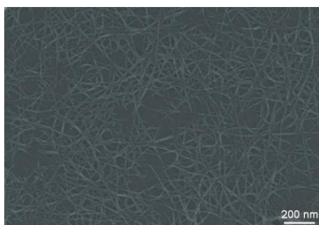
Fig. S7. The typical SEM image of purified iron-etched SWNTs
