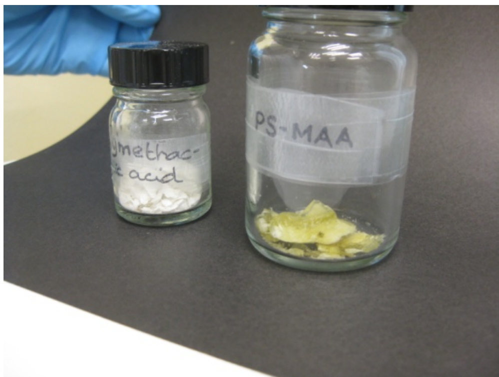
Figure S9. (a). PMAA and (b). PMAA- b /ran-PS (as collected from the reaction flask after the reaction).
