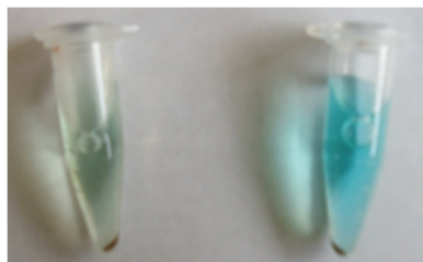
Figure S7. Tubes containing free SC (left) and SC -stained nanoparticles (right) after 45 min incubation with red blood cells and pelleting of the cells by centrifugation. The cells extracted most of the blue-colored SC from the solution but not the SC -stained nanoparticles
