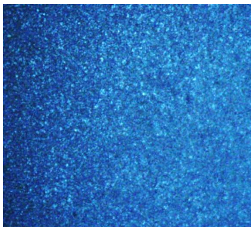
Figure S4. The original POM picture of 1 under crossed polarizers recorded upon cooling to RT from melt at a rate of 2\text{ }^{\circ}\text{C min}^{-1} .
