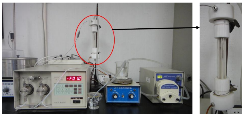
Figure S1. Digital photos of GBMR device. The right photo is the ceramic membrane reactor composed of four ceramic membrane tubes, which is the core of the device of GBMR method.
