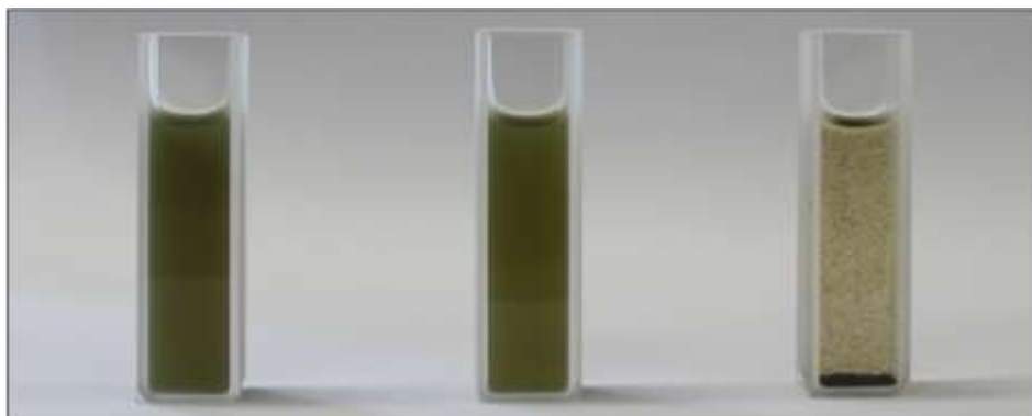
Fig. S4 Photograph of a MoS 2 /GO/PEO (6/3/1) system before (left) and after (middle) coordination, and a MoS 2 /GO (6/3) system after coordination for comparison (right).
