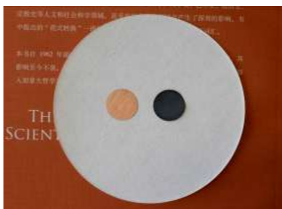
Fig. S9 Photograph of a naked copper foil (left) and a copper foil attached with the tailored freestanding \text{MoS}_2/r\text{-GO/PEO} (6/3/1) hybrid paper (right). Note that there is still scope for improving the electrochemical performance of our film anode by, e.g. , rationally reducing its thickness to shorten the diffusion pathways, or trying to further optimise its composition.
