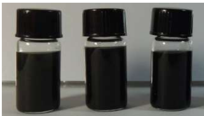
Fig. S7 Photograph of three coordinated MoS 2 /r-GO/PEO systems (7/2/1, 6/3/1 and 5/4/1).
