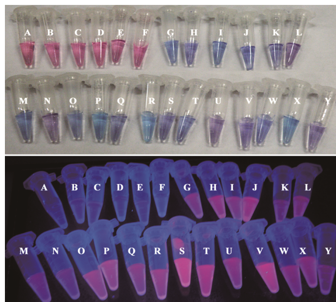
Figure S10. Photograph (taken under ambient light or UV light) of 5 \mu\text{M} ISCH-1 without (A) and with 5 \mu\text{M} dA21 (B), dT21 (C), CT-DNA (D), ds15 (E), BSA (F), c-kit1 (G), bcl-2 (H), pu27 (I), THTG (J), VEGF (K), Rb (L), c-kit2 (M), RET (N), ILPR (O), KRAS (P), STAT3 (Q), pu18 (R), htg21 (S), dimer (T), tetramer (U), HT-6 (V), rDNA-2957 (W), rDNA-5701 (X), rDNA-13079 (Y).
