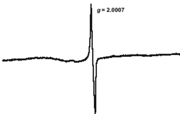
Fig. S10 EPR spectrum of \text{PBCE}\cdot\text{Li}^+\text{@C}_{60} in PhCN showing the radical ion with corresponding g value at 77 K observed after photoirradiation.
