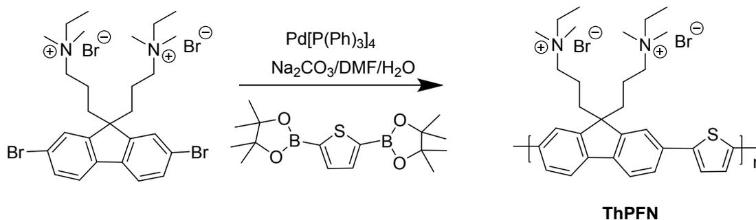
**Scheme S1.** Schematic preparation and molecular structure of the conjugated polymer ThPFN.
