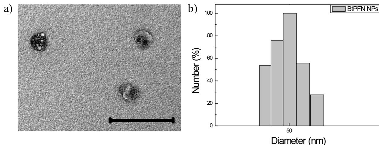
**Figure S1.** a) TEM image and b) hydrodynamic diameter distribution of BtPFN NPs. (Scale bar: 200 nm)
