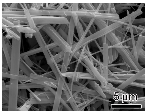
Fig. S4. SEM image of the product synthesized with \text{Na}_2\text{C}_2\text{O}_4/\text{TiO}_2 molar ratio of 1 : 2 in the absence of surfactant NP-9.
