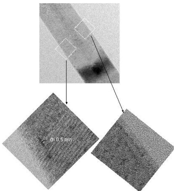
Figure S8. HRTEM image of VO<sub>2</sub> nanoribbon, showing V<sub>3</sub>O<sub>7</sub> phase due to surface oxidation after exposure of the sample to air
