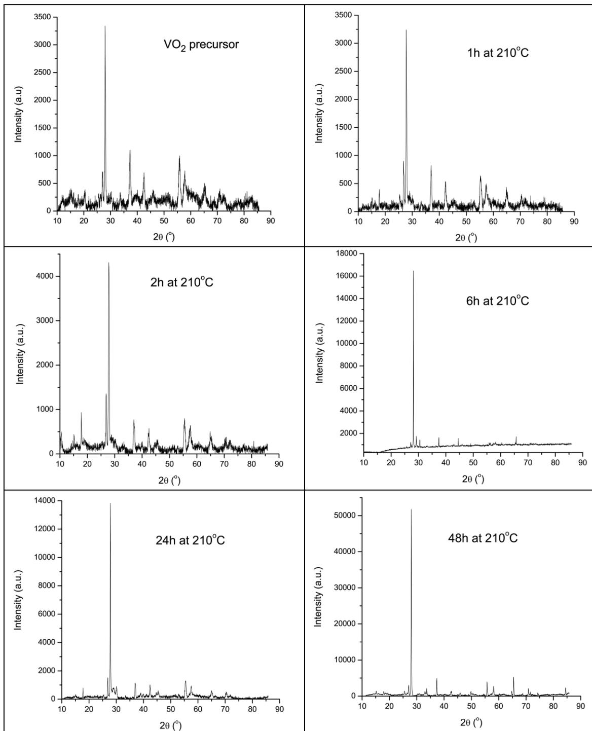
Figure S1. XRD spectra of products of ligand-free reactions of hydrothermal VO<sub>2</sub> (M) nanoribbon synthesis after different reaction times
