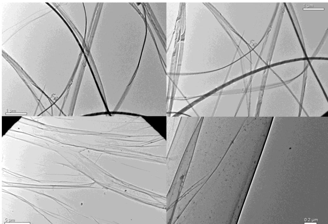
Figure S6. TEM images of VO<sub>2</sub> nanostructures produced in hydrothermal reaction with acetone as a ligand (top: 30 μl; bottom: 200 μl)
