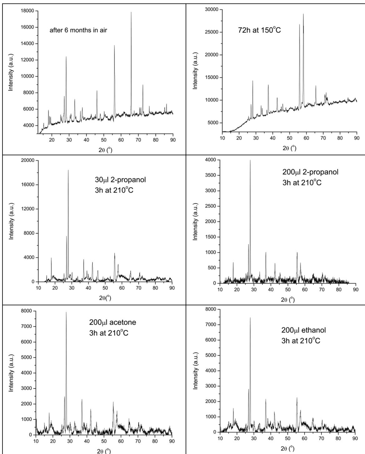
Figure S2. XRD of products of hydrothermal synthesis of  $\text{VO}_2$  (M) nanocrystals synthesized under different reaction conditions and using different ligand molecules
