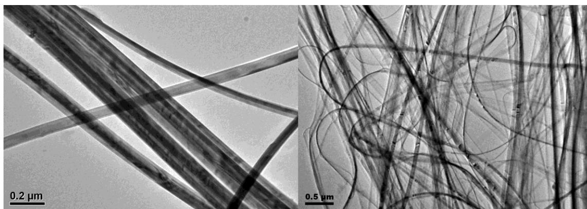
Figure S5. TEM images of VO<sub>2</sub> nanostructures produced in hydrothermal reaction with 2-propanol as a ligand (left: 30 μl; right: 200 μl)
