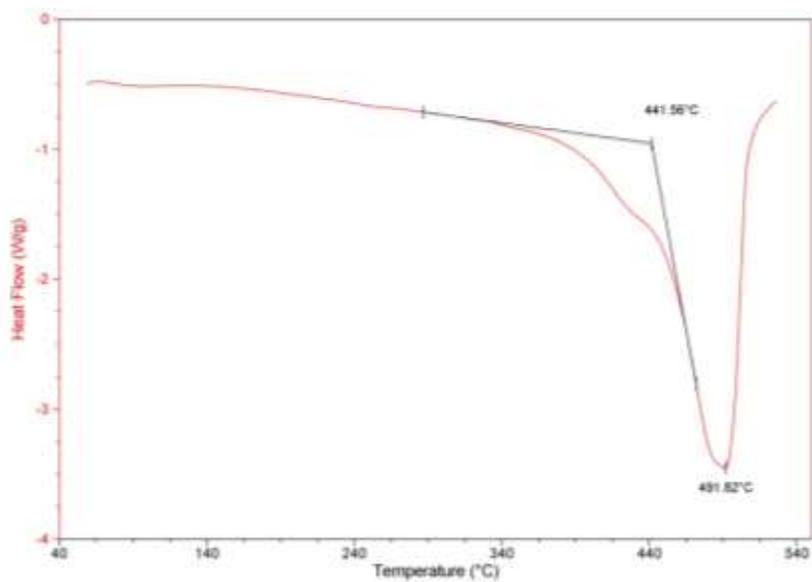
DSC curve of MgBA<sub>2</sub> (sealed pan).
