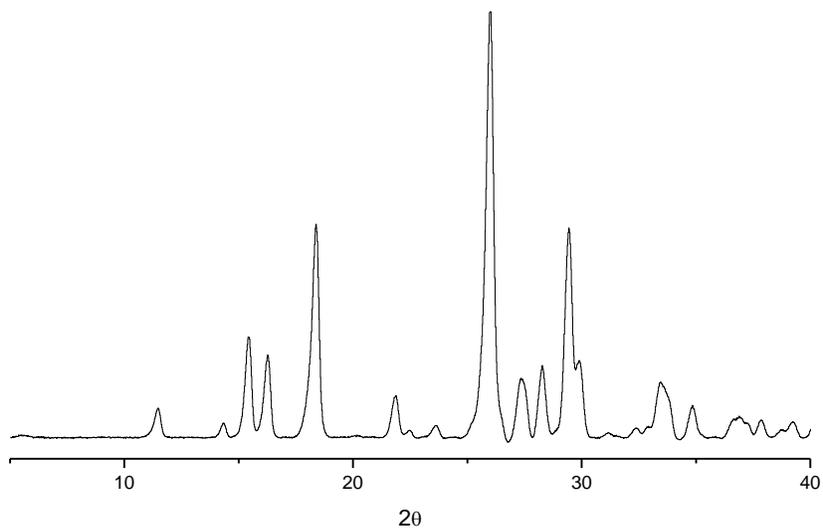
Experimental pattern of  $\text{MgBA}_2 \cdot 2\text{H}_2\text{O}$
