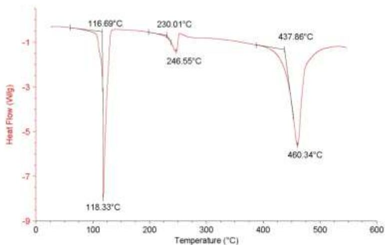
DSC curve of NaBA·HBA·2H<sub>2</sub>O (sealed pan).
