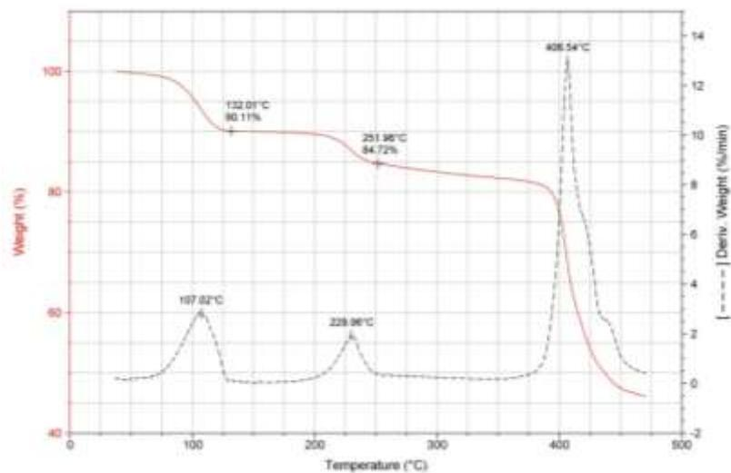
TGA curve of KBA·HBA<sub>0.5</sub>·1.5H<sub>2</sub>O.
