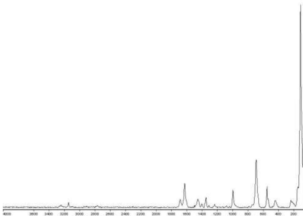
Raman spectrum of the salt  $\text{MgBA}_2 \cdot 2\text{H}_2\text{O}$ .
