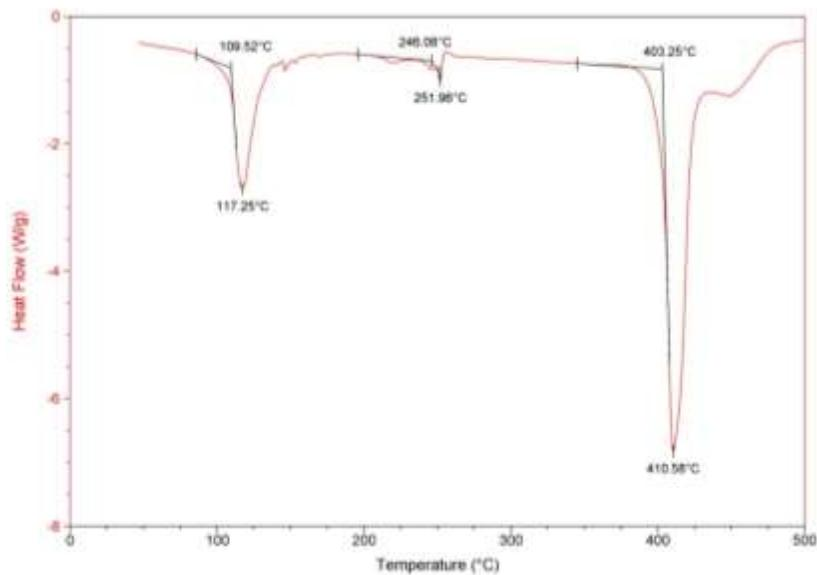
DSC curve of KBA·HBA<sub>0.5</sub>·1.5H<sub>2</sub>O (sealed pan).
