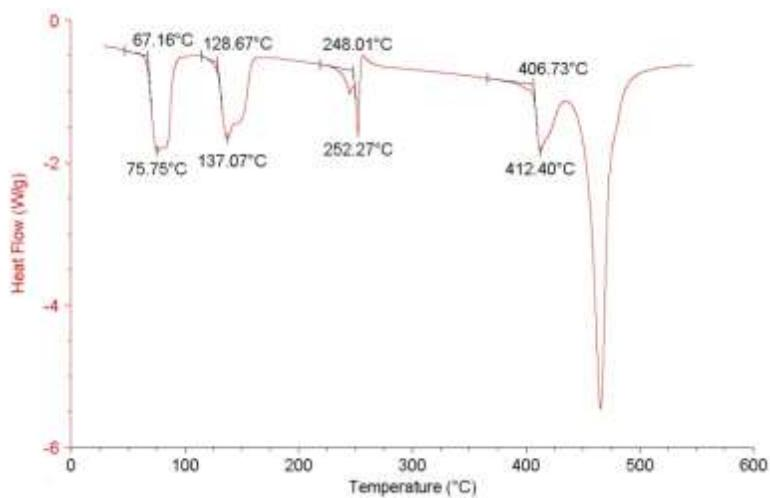
DSC curve of KBA·HBA·2H<sub>2</sub>O (sealed pan).
