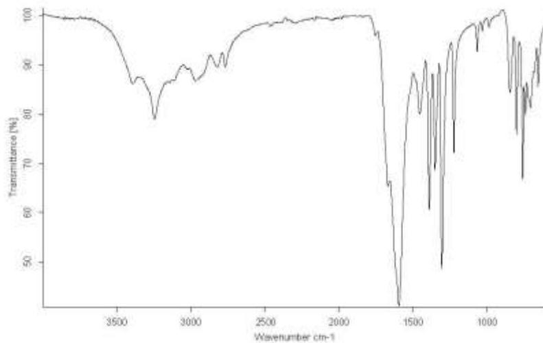
IR (ATR) spectrum of MgBA<sub>2</sub>·2H<sub>2</sub>O
