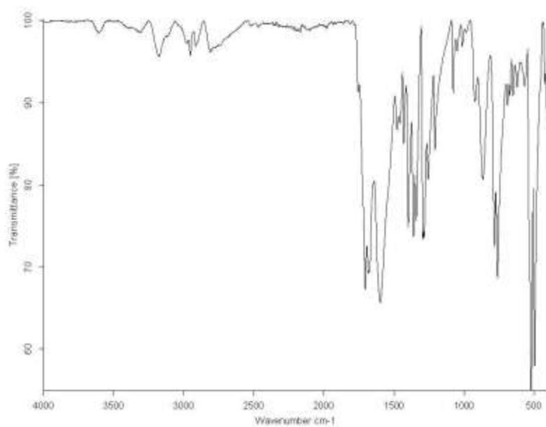
IR (ATR) spectrum of  $\text{KBA}\cdot\text{HBA}_{0.5}\cdot 1.5\text{H}_2\text{O}$ .
