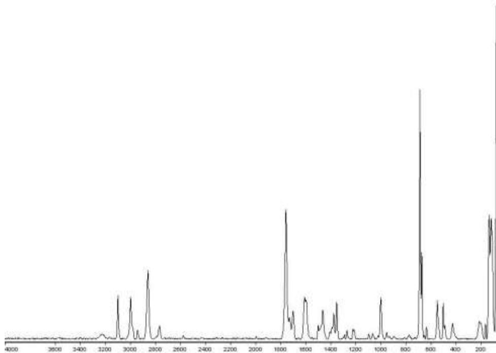
Raman spectrum of the salt co-crystal NaBA·HBA·2H<sub>2</sub>O.
