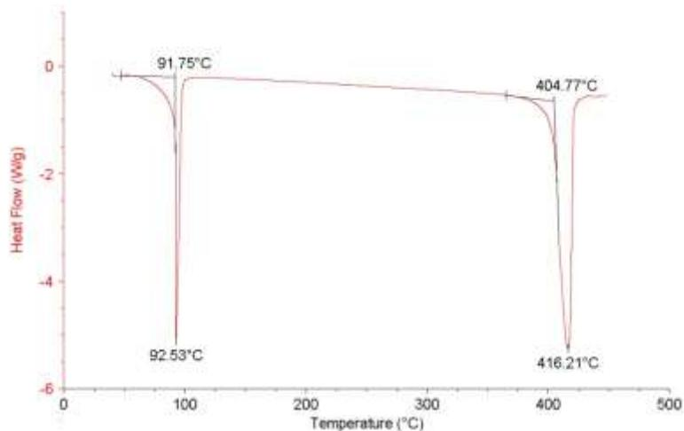
DSC curve of NaBA·1H<sub>2</sub>O (sealed pan).
