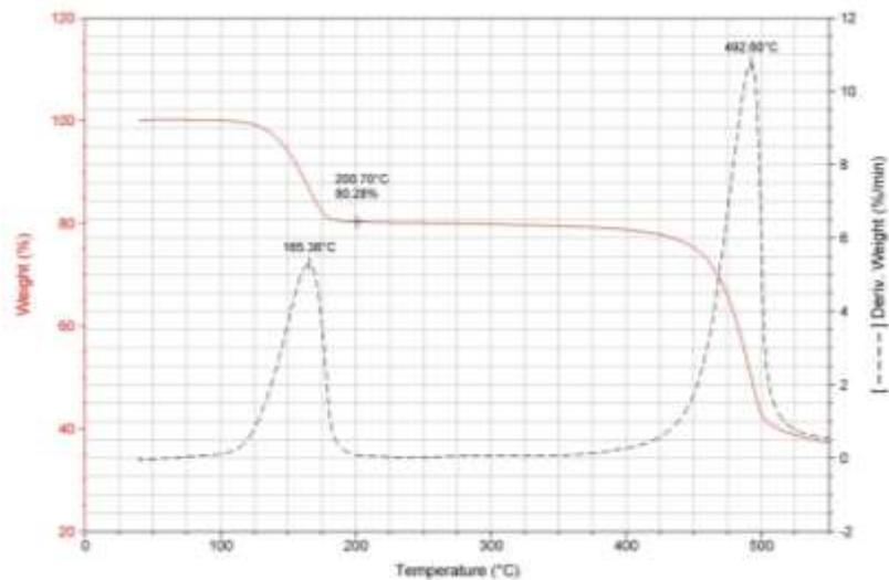
TGA curve of MgBA<sub>2</sub>·2H<sub>2</sub>O
