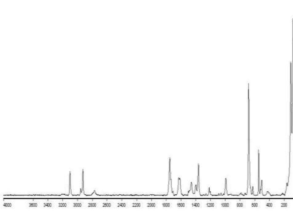
Raman spectrum of the salt co-crystal  $\text{KBA} \cdot \text{HBA}_{0.5} \cdot 1.5\text{H}_2\text{O}$ .
