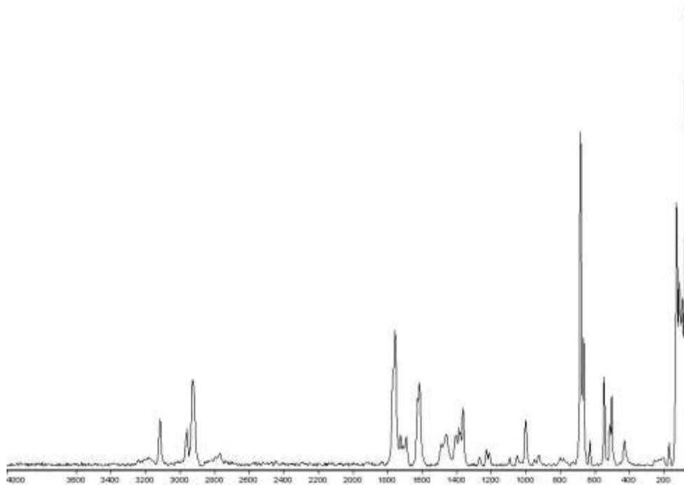
Raman spectrum of the salt co-crystal  $\text{KBA} \cdot \text{HBA} \cdot 2\text{H}_2\text{O}$ .
