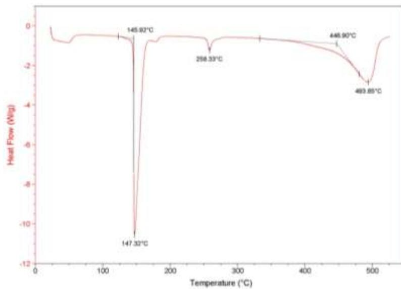
DSC curve of MgBA<sub>2</sub>·2H<sub>2</sub>O (sealed pan).
