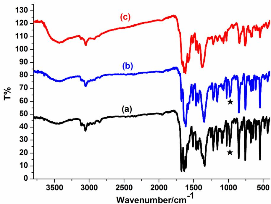
Fig.S3 IR spectra of **1** (a), desolventized sample **1'** (b), and irradiated sample **1-i** (c).
