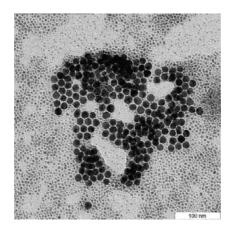
**Figure S1.** TEM image of a Ag/Au NP bilayer, obtained by sonicating them for 1 h after transferred from the water/toluene interface. The black large dots are 12 nm Au NPs while the grey small dots 6 nm Ag NPs. The sonication caused detachment of the Au NPs rather than Ag NPs, suggesting a bilayer character of the resulting films.
