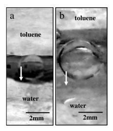
**Figure S2.** Photographs of water droplets of 20  $\mu$ L and 200  $\mu$ L in volume, standing on a Ag/Au NP bilayer (a) and a Ag/Au/CdTe NP trilayer (b), self-assembled at the water/toluene interface. The upper phase is toluene and the lower phase water. The interface is highlighted by arrows.
