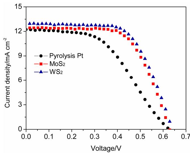
**Fig. S3** Photocurrent density-voltage ( $J$ - $V$ ) curves of the  $\text{T}_2/\text{T}^-$  based DSCs using Pt,  $\text{MoS}_2$  and  $\text{WS}_2$  CEs.
