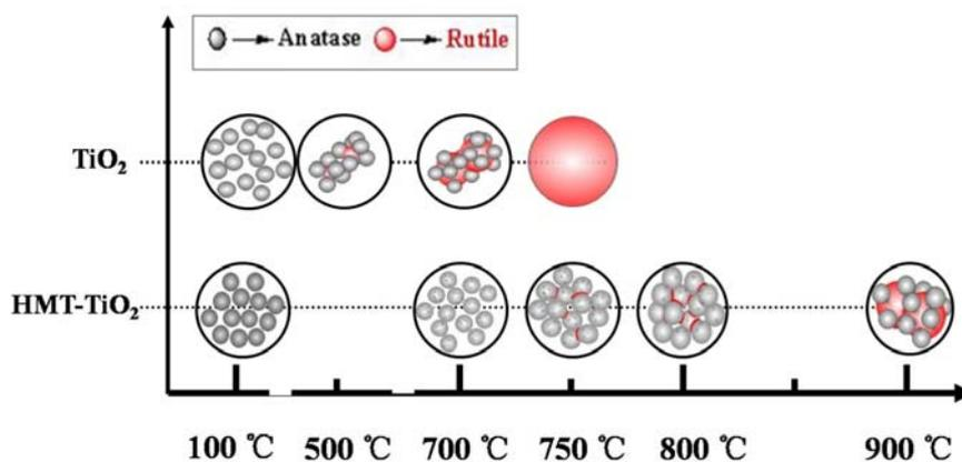
**SI-figure 5. XRD patterns of different TiO<sub>2</sub> samples by sol-gel process**
