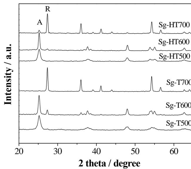
**SI-figure 6. XRD patterns of TiO<sub>2</sub> samples modified by ammonia**
