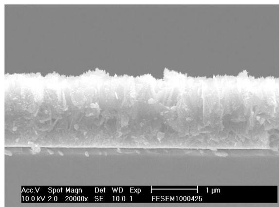
Fig. S1 Cross-sectional-view SEM image of ZnO nanosheet framework.
