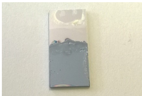
Figure S4: Photograph of the germanium film electrodeposited at -0.9 V at 180 °C for one hour. The counter electrode was a p -type germanium wafer. The solution was stirred by a magnetic stirrer bar.
