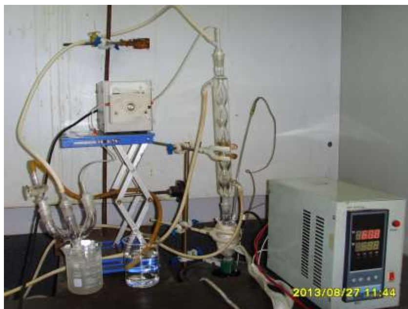
Figure S1. Photograph of the Reactive Distillation Column setup.
