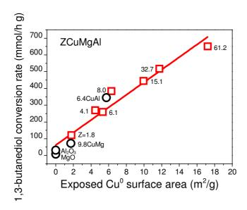
Linear relationship between the amount of exposed Cu<sup>0</sup> species and the 1,3-butanediol overall reaction rate on ZCuMgAl, 9.8CuMg, 6.4CuAl, MgO and Al<sub>2</sub>O<sub>3</sub> catalysts [T = 523K;  $\bar{P}_{BDO} = 2.33kPa$ ]
