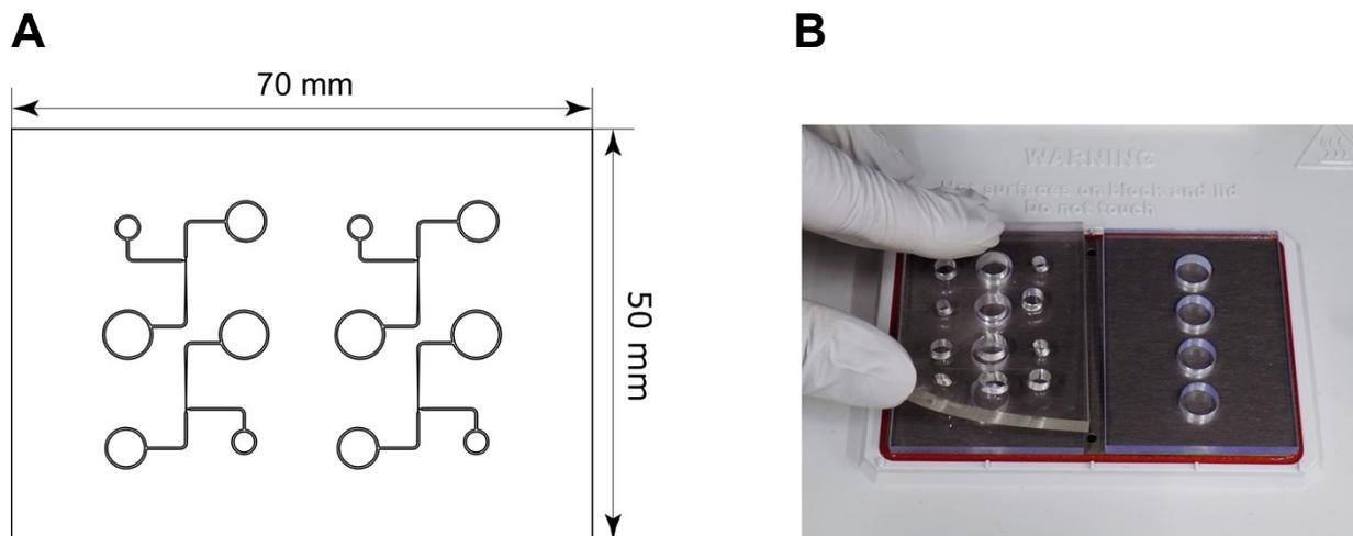
(A) Schematic drawing of the four identical inlet/outlet systems configured on the single cartridge and (B) photograph of the two cartridges on the heating block of the thermocycler.
