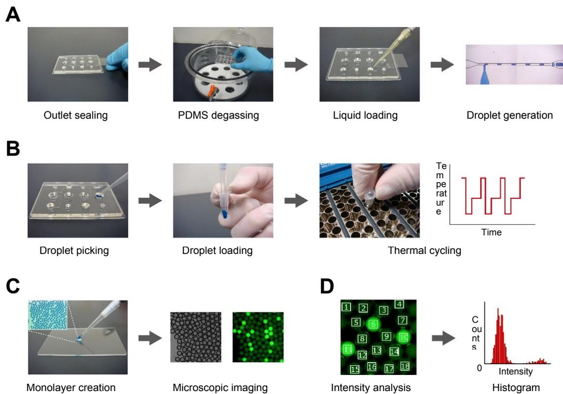
The sequential experimental procedures in the previous droplet PCR study<sup>1</sup> are schematically shown. (A) Automatic droplet creation, (B) PCR, (C) droplet imaging, and (D) data analysis. For clarity of display, a blue food dye solution was used as the aqueous phase. Adapted with permission from *Electrophoresis*, 2017, **38**, 296–304 (<https://doi.org/10.1002/elps.201600309>).<sup>1</sup>
