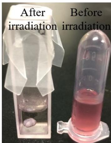
**Figure S4.** The digital images of the solution of Au NPs (50 nm) before and after irradiation with 680 nm laser for a cycle of heating.
