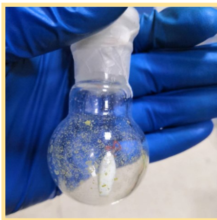
Figure S16. The resulting electrolyte was concentrated in a decompression distillation plant after electrolysis at a potential of -0.1 V (vs. RHE).
