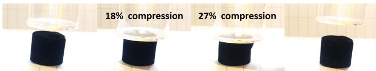
**Fig. S5** A simple compressibility test of the MgAl-MMO/rCNT aerogel under vial compression.
