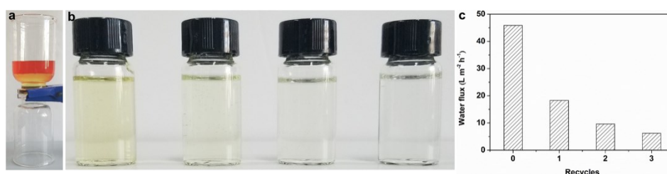
Fig. S9 The pore clogging experiments for traditional filtration. (a) The water pre-wetted superhydrophilic PP patterned membrane (pore size: 0.22 \mu\text{m} ) separates the hexane (dyed by Oil Red)-water (Fast Blue BB salt solution, yellow) mixture (50 mL-50 mL) by traditional filtration method. The colour of filtrates (b) before filtration (original solution) and after filtration with different recycles (1, 2, 3) for traditional filtration. (d) The flux of traditional filtration with increased recycles.
