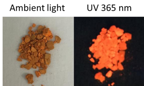
Figure S2 Photographs of the complex 1-Pt under ambient light and under UV light (365 nm).
