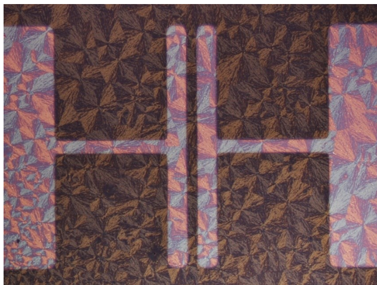
Figure S23. Polarized light microscopy image of dDTCB thin film coated on glass substrate with source and drain electrodes after annealing at 100 °C for 10 min.
