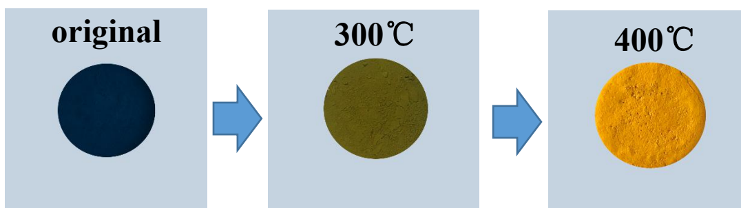
Figure S16. (a)When the sample is heated in air at 300 °C and 400 °C for 5 h, with the decrease of V_o , the sample finally becomes V_2O_5 .
