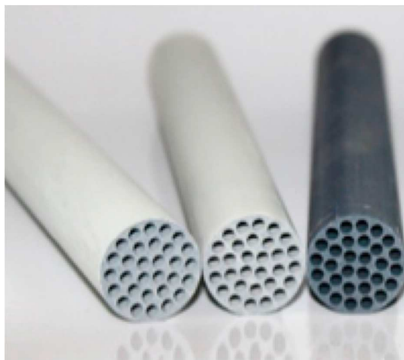
Figure S2. Picture of SiC monolith structures used in the present work.
