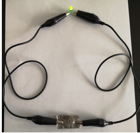
Fig. S7. Demonstration of a green LED powered up by NiFe 2 O 4 @Ni-Mn LDH/NF//AC ASC.
