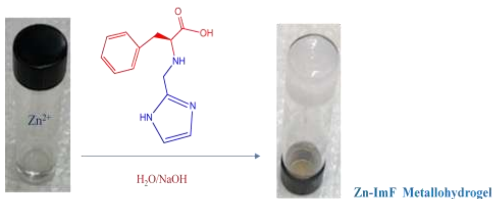
Fig. S13. Molecular structure of the ImF gelator and the formation of the Zn-ImF metallohydrogel in a 2:1 ImF:Zn 2+ mole ratio.
