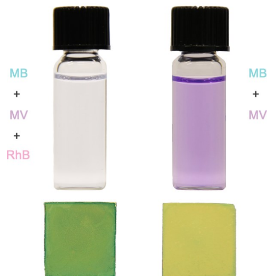
Figure S13 Colours of PTA@HKUST-1 SURMOF (bottom) after being immersed in the dye mixtures and colours of 25 mM \text{NH}_4\text{Cl} ethanol-water solutions (top, the volume ratio of ethanol/water is 160) after soaking of the dye loaded PTA@HKUST-1 SURMOF, indicating the selective adsorption feature of PTA@HKUST-1 SURMOF.
