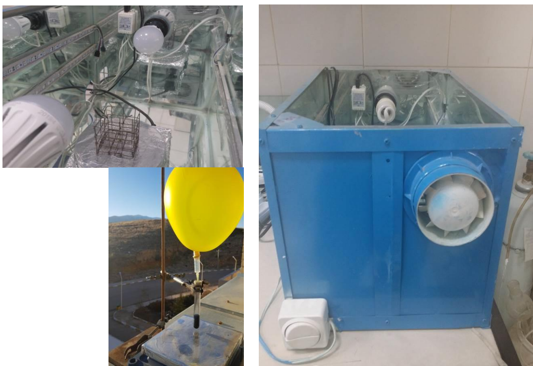
Figure S1. The box containing 15 W blue LED lamp ( \lambda > 410 nm) and the reaction setup up under sunlight.
